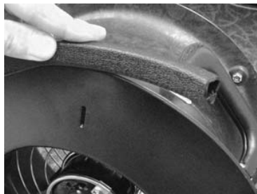
Figure 3-8: Transition piece holding flow ring onto fan
